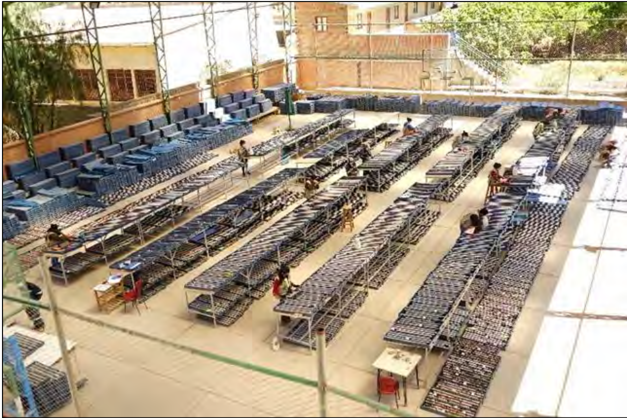
Figure 10.8 Drill Core Logging and Sampling Facilities at Iska Iska
